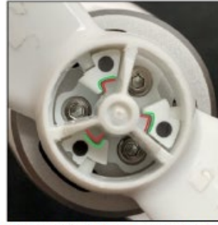
Figure 12. Lugs and Notches on the Phantom 4 (after engagement) (CPX-0021)
