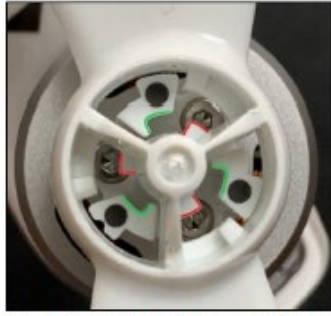
Figure 11. Lugs and Notches on the Phantom 4 (before engagement) (CPX-0021)
