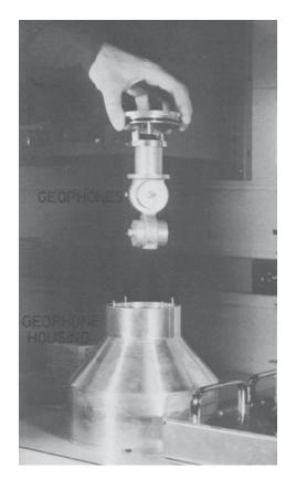
Appx1262, Appx1263 ("The three geophones are mounted in a single aluminum frame and suspended from a gimbal joint in viscous oil. The gimbal ensures vertical seismometer orientation for instrument tilts up to 30°..."); see also Appx2772 at ¶ 89.
