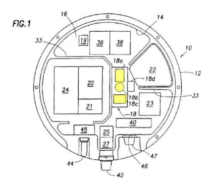
Appx680 at Fig. 1, Appx684 at 6:43-49 ("It will be further noted that geophone 18 is internally mounted within pod 10 and thus requires no external wiring or connection. It has been determined that utilizing a compact case and positioning geophone 18 adjacent the casing wall, geophone 18 can be effectively coupled to the earth such that seismic data transmitted through pod 10 to geophone 18 is not corrupted by interference.").
