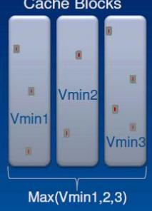
The diagram illustrates three cache blocks. Each block contains several small red squares representing cache cells. The first block is labeled  $V_{min1}$ , the second  $V_{min2}$ , and the third  $V_{min3}$ . A bracket below the blocks indicates the maximum voltage level as  $Max(V_{min1,2,3})$ .
