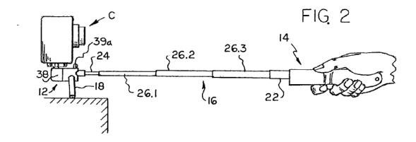
Fromm Figure 2, above, shows an extensible telescoping support 16 that extends between a base assembly 12, where a camera is secured, and a handgrip 14. Ex. 1010, 1:15–25. A battery powered remote control device, e.g., one integrated into the handle, allows the user to activate a zoom, shutter release, and playback from the remote control using communication codes, e.g., infrared codes. *Id.* at 7:54–8:11.
