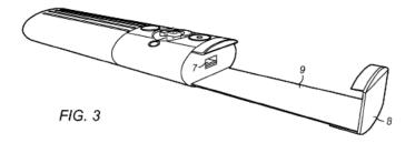
Figure 3 illustrates the handle's sliding plate. *Id.* at 2:7–8. The handle base module includes transformable chuck 8, sliding plate 9, a magnet and spring (not shown), button 1 (not shown) used to open and close sliding plate 9 to fix the position of the handheld terminal and transformable chuck 8. *Id.* at 3:31–37; 4:1–9.
