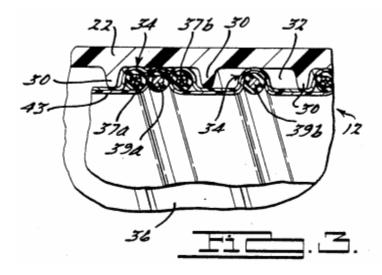
Figure 3 is a cross-sectional end view of the handle assembly of Rohn. *Id.* The inner surface of first handle section 22 includes a number of annular, parallel, ridge portions 30 integrally formed in a longitudinal, annular, groove-like channel section 32 of the first handle section 22. *Id.* at 3:10–14. Channel section 32 generally holds an elbow section (not shown in Figure 3) and a portion of the vacuum hose 12 therein. *Id.* at 3:14–16.
