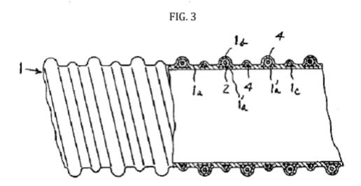
Figure 3 of Nagayoshi depicts resin-covered steel wire 2, which is formed by being covered with a soft-synthetic-resin covering layer 1a' forming an inner periphery wall surface of the tube wall 1a. *Id.* at 4:27–32
