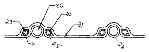
Figure 3 depicts a cut-away view of one embodiment of the hose of the '127 patent. *Id.* at 3:29–30. In this embodiment, there are insulated conductor wires 24 and 25 on opposite sides of structural helix 22. *Id.* at 4:43–47.
