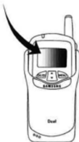
*Id.* (annotated figure). The display screen also includes a backlight. *Id.*, pp. 16, 38, 42. Samsung explains that a user can select various backlight options, including “Flip Open, 10 or 30 Seconds (after last keypress), or Off.” *Id.*, pp. 42, 96.
