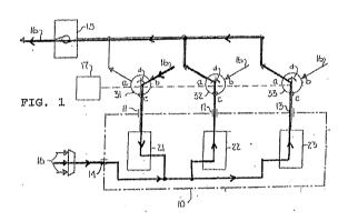
vacuum machine. This air enters the canister 10, passing through a series of filters 21, 22, 23, each of which is connected to an outlet port 11, 12, 13. A valve 31, 32, 33 is connected to each outlet port 11, 12, 13. Each valve 31, 32, 33 has ports 31a, 32a, 33a that communicate with the vacuum source 15, and ports 31b, 32b, 33b
