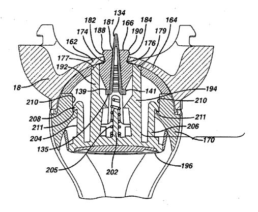
Ex. 1, '077 Patent, Fig. 39. As shown above, the latches 162, 164 engage the handle and prevent slippage of the cartridge from the handle.
