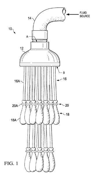
In the embodiment that appears to be claimed in claim 1, depicted in Figure 1 (reproduced above) (Appx47), the system (10) includes a housing (12) attached to a hose (14) at end A and to hollow tubes (16) at end B. Appx53 (col. 2, ll. 35-37). Containers, *e.g.*, balloons (18), are clamped to the tubes (16) using elastic fasteners (20) such as O-rings, which regulate fluid flow by opening, closing, or partially obstructing fluid passageways. *Id.* (col. 2, ll. 51-57).
