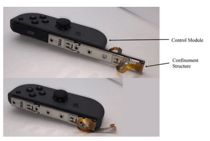
1(f) (i) and in which the structural bridge comprising: a conduit between the pair of control modules; The structural bridge in the Nintendo Switch comprises a pathway between the two Joy-Cons.
