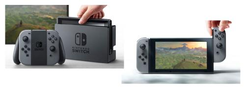
when mobility is desired, users can remove the gaming console from its dock and attach the two Joy Con controllers to rails on each side of the Switch console, creating a mobile, handheld gaming device.
