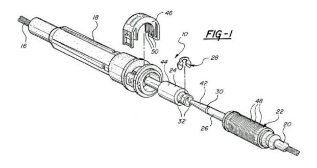
The '953 patent is directed to a "Molded Terminal with Vibration Dampener Pocket." The '953 patent describes an invention that allows for attachment of the shift cable to the shift knob and the transmission in a manner that minimizes noise and vibration transmitted from the transmission to the shift knob.
